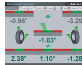
Real-time indicators to verify measurements after adjustment
